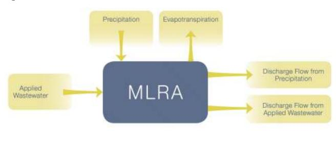
Figure 2-2: LAS Water Balance Schematic
