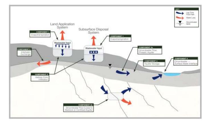
Figure 2-1: Conceptual Model of Flow from Wastewater Disposal Systems to Surface Water
