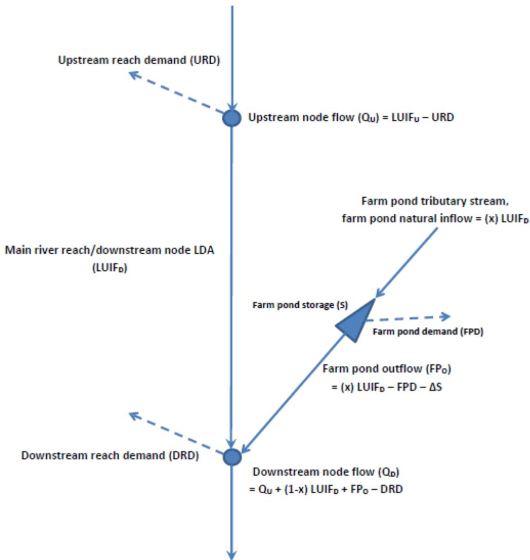
Figure 5-7 Conceptual surface runoff-supplied farm pond resource assessment model schematic
