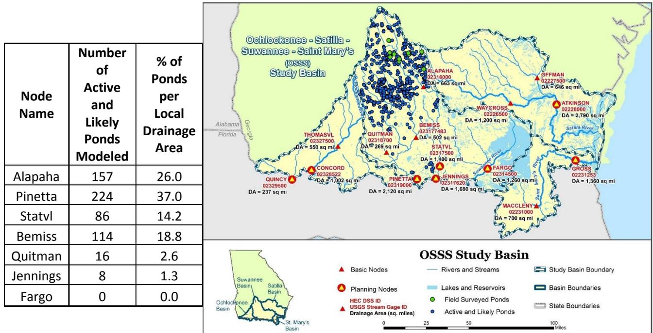
Figure 5-2 Suwannee River Basin (OSSS Study Basin) showing active and likely farm pond locations (dark blue dots) and field surveyed farm ponds (10 – green dots )
