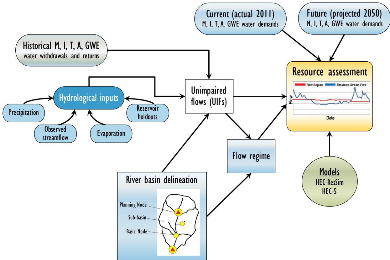
**Figure 1-1 Surface water availability resource assessment process components**
