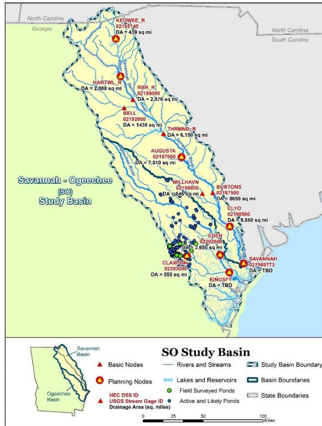
Figure 5-3 Ogeechee River Basin (SO Study Basin) showing active and likely farm pond locations (dark blue dots) and field surveyed farm ponds (10 – green dots)
