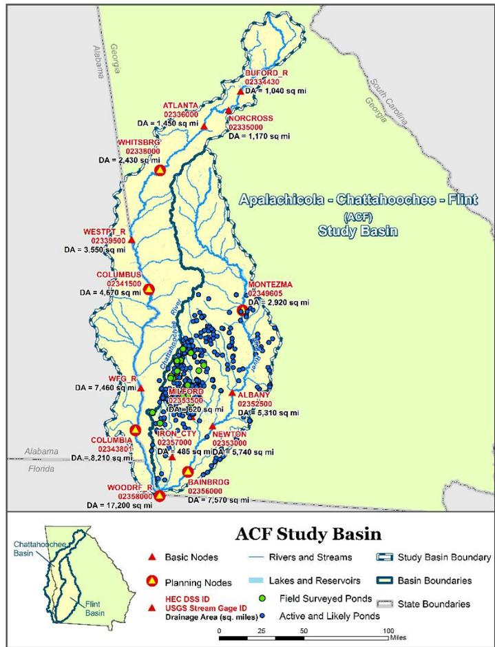
Figure 5-1 Flint River (ACF Study Basin) showing active and likely farm pond locations (dark blue dots) and field surveyed farm ponds (20 – green dots)
