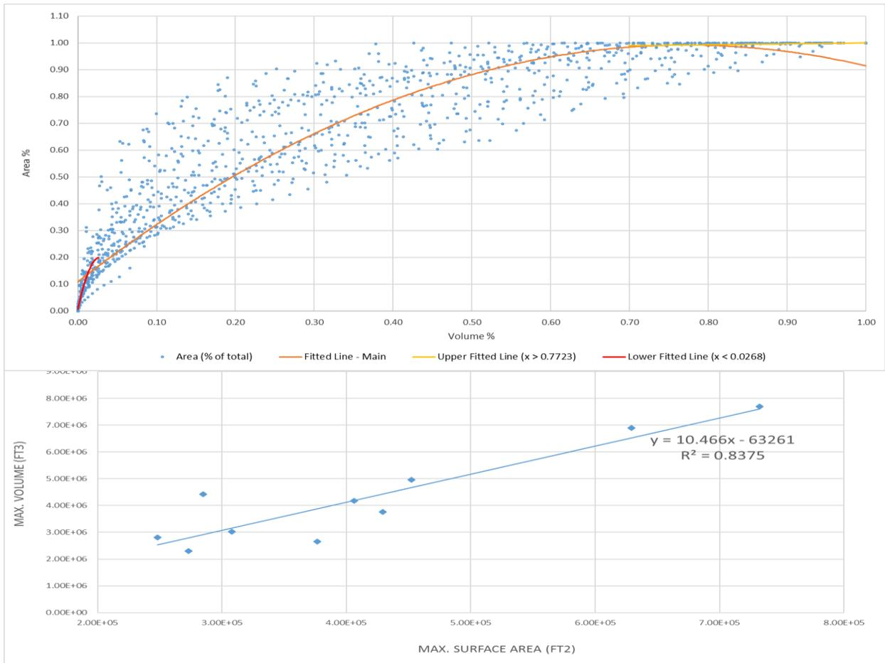
**Figure 5-6 Best-fit dimensionless storage-area and maximum storage-area relationships for surveyed farm ponds in the Ogeechee River Basin**
