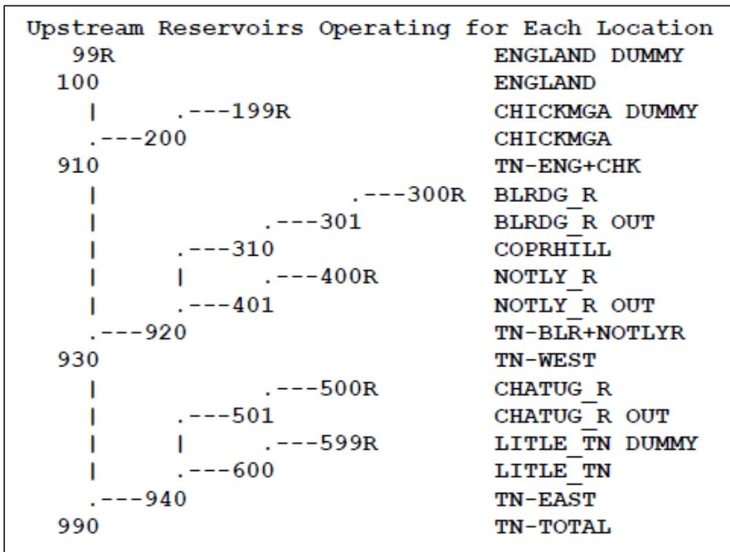
Figure 6-13 TN HEC-5 resource assessment model system connectivity diagram
