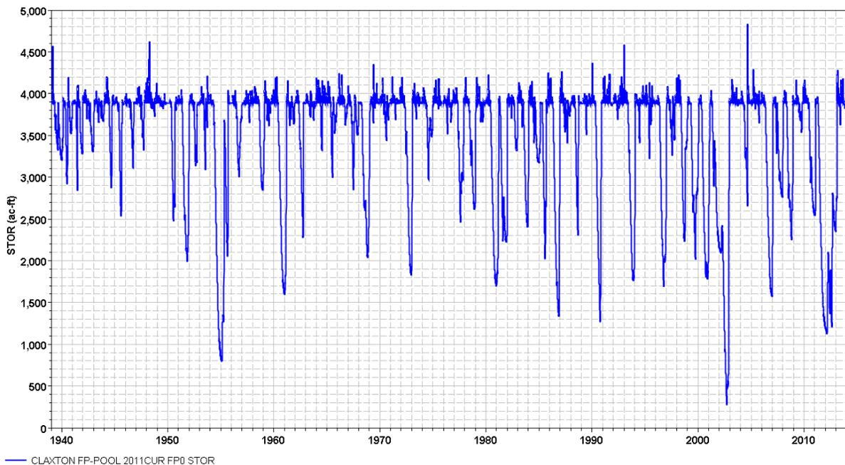
**Figure 5-8** Example simulated surface runoff-supplied composite farm pond storage utilization with current (2011) water use, Canoochee River Basin above Claxton (SO Study Basin)
