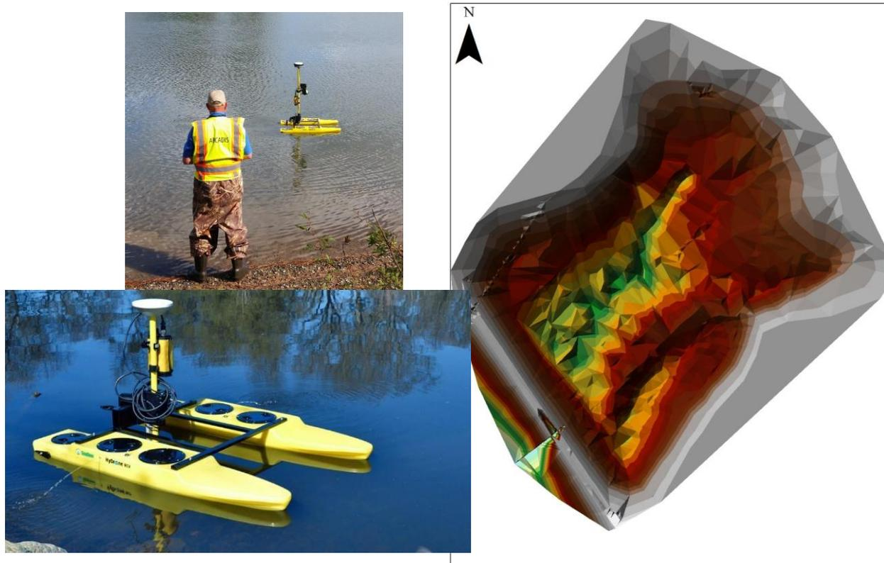
Figure 5-5 Bathymetric survey equipment and resulting farm pond digital elevation model
