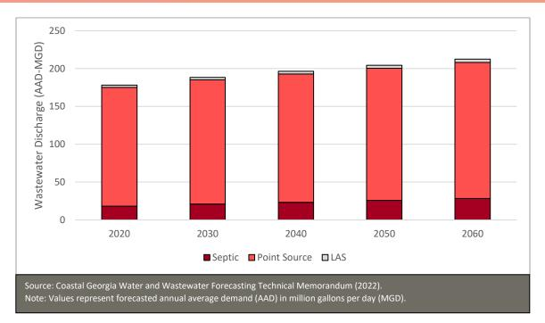
Figure 4-6 Total Wastewater Forecast (in AAD-MGD)
