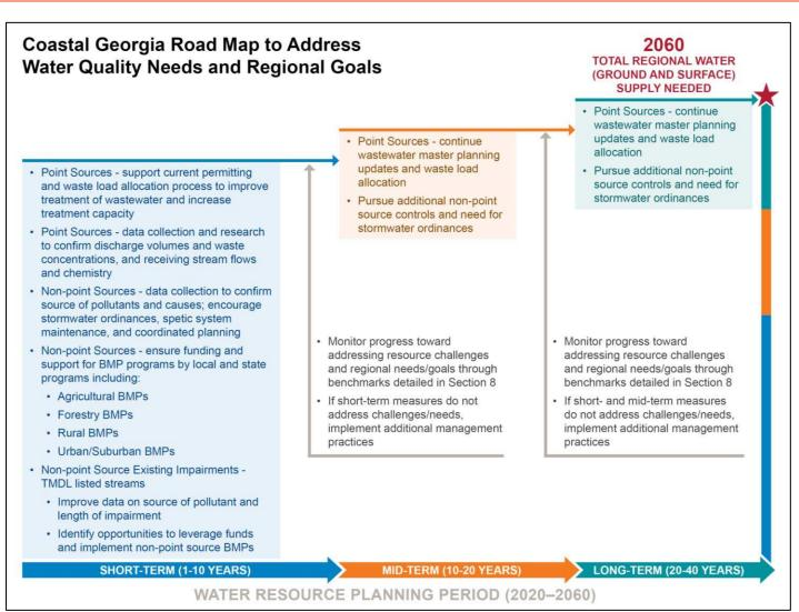
Figure 6-2 Recommended Surface Water Quality Management Practices in a Phased Approach
