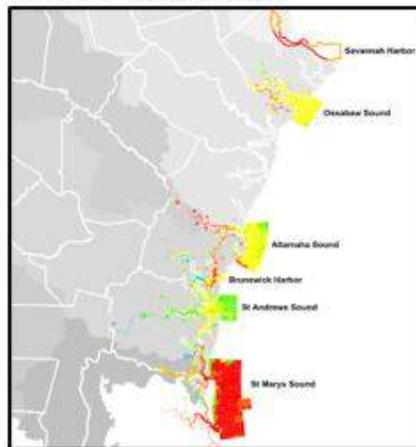
Figure 3-6 Results of Assimilative Capacity Assessment – DO Under Current Permit Conditions
